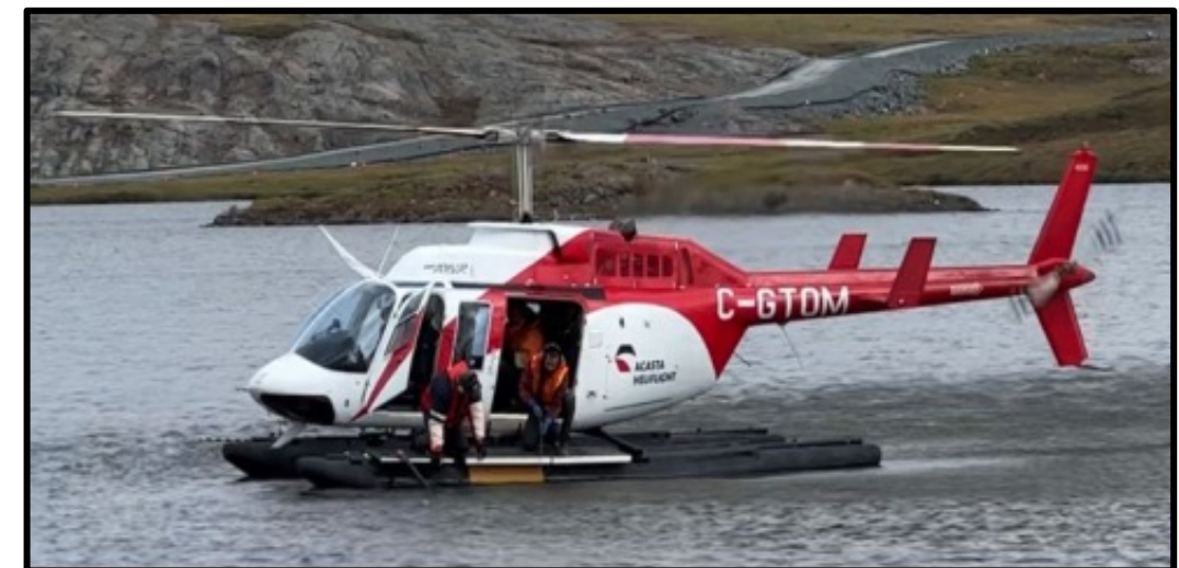
Lake Sediment Sampling – using torpedo off side of helicopter with floats
